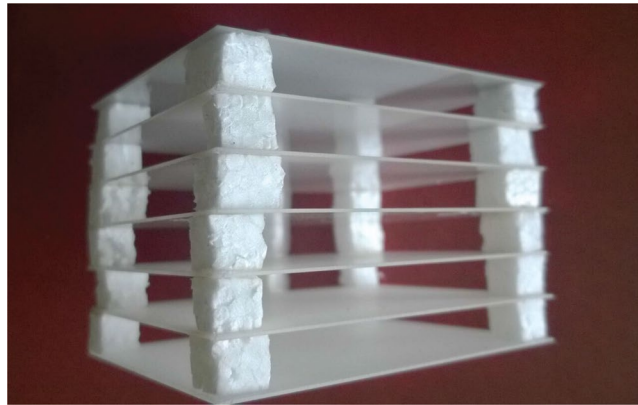
Figure 2. One dimensional photonic crystal. Photograph of the 1d PC used in the experiment. It is formed from 7 alumina ceramic plates with \varepsilon = 10 , thickness b = 0.5 mm, sizes 60 \times 96 mm 2 and a = 10 mm distance from each other.
