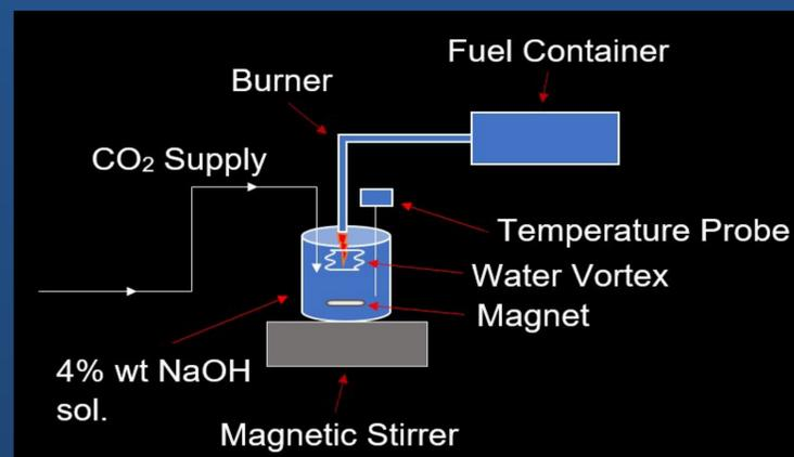
Conversion of aqueous NaOH solution into Na<sub>2</sub>CO<sub>3</sub> precipitate and steam via utilization of available CO<sub>2</sub> and direct contact heat transfer mechanism
