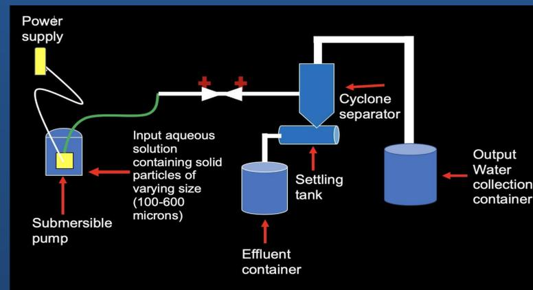
Cyclone separation-based decantation of solid particles from aqueous solutions
