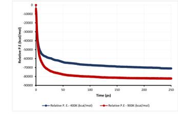
The 900 K simulation released more energy (almost 20,000 kcal/mol at and after 50 ps) and separated more oxygen (at least 50 more O<sub>2</sub> molecules) than at 400 K. So 900 K is a more effective temperature for ANP fuel and will be used in our water and methane cases.
