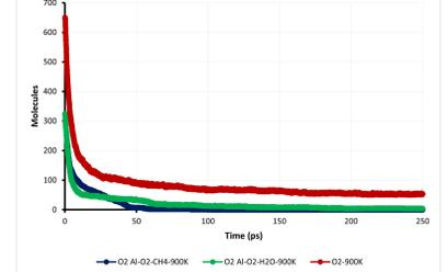
The greatest energy released from our ANP combustion MD simulations was with the oxygen at 900 K case, where the greatest access to oxygen had the best oxidation of the ANP (greatest amount of O<sub>2</sub> separation). Oxygen-water combustion with ANP released less energy, but released more than the combustion with oxygen-methane.
