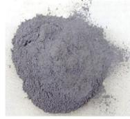
Ex. of ANPs, aluminum nanoparticle dust.<sup>10</sup>
