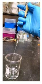
3. *Gently release the bulb to draw the liquid into the pipet.* Do not draw liquid into the bulb or the top segment of the pipet. If you notice that the liquid squirts out of the bottom of the pipet, pull in and then expel the liquid several times.
