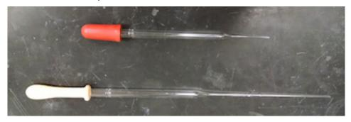
2. *Squeeze the bulb and then insert the tip of the pipet into the liquid you wish to transfer.* Be sure to hold the pipet in an upright position.
