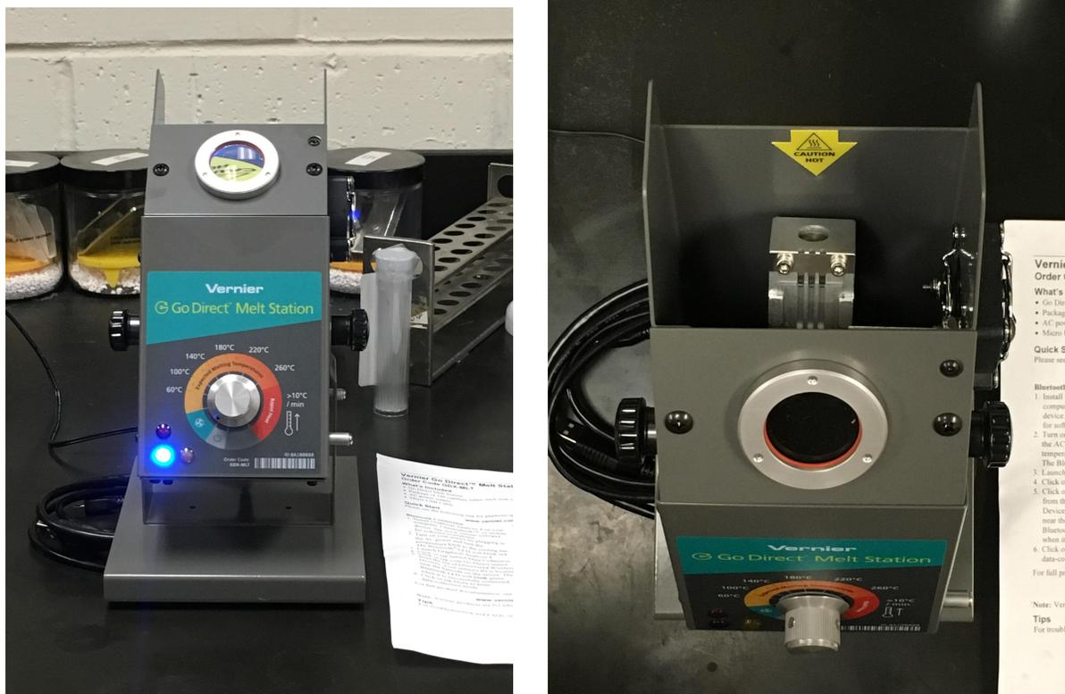
Figure 1: Front view of Vernier Go Direct Melt Station (left) and top view showing sample holder (right).
